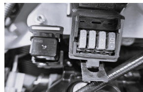
Fuse Box with Cover open
