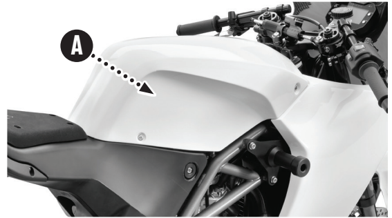
Intake Cover / Air Filter Box
